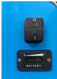
Always ensure the GB Compact has been adequately charged by checking the battery level.
