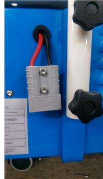
Connect the charger to the GB Compact using the socket at the rear of the machine.
