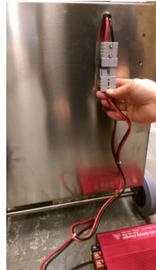
Connect the charger to the GB1 using the socket at the rear of the machine.
