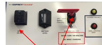
Turn the Isolator switch to the ON position and press the Boiler ON button once.
