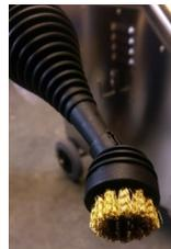
Ensure the brass brush is adequate for work, if not, remove & replace
