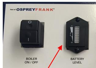
Always ensure the GB1 has been adequately charged by checking the battery level. Green indicates adequate batter charge, red indicates low battery. Failure to fully charge the unit will result in a shortened working day
