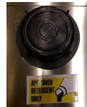
Unscrew the black detergent tank lid and fill with the GumBusters chewing gum detergent and cold clean tap water (10litres) \*
