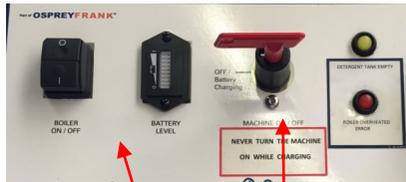
Ensure the Machine ON/OFF switch & the BOILER switches are both in the OFF position and no light is showing for the battery level.
