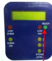
Allow 9 mins for the machine to heat up. The machine is ready when the Green Indicator light illuminates
