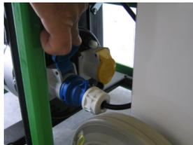
Connect machine plug to generator socket
