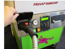
Open the front panel and connect the steam hose with the red button facing up. Push firmly and the hose will click into place
