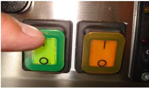
Plug machine into a suitable electric socket and press top section of green on/off switch
