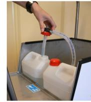
Remove Red water reservoir cap and fill with clean cold tap water. Fill 2nd reservoir if required and close lid
