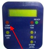
This light, when illuminated, indicates the chemical tank needs refilling
