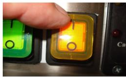
After a few seconds press top section of Orange Boiler switch
