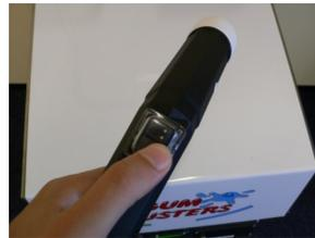
Use left switch to activate chemical Injection. Detergent pump will dose automatically every second
