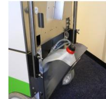
Open chemical container compartment at the rear and fill with manufacturers approved chemical if required
