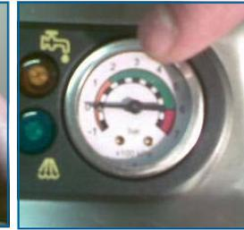
De-pressure the boiler: Press the left switch of the pistol grip and the trigger (red switch underneath the pistol grip), until the pressure gauge shows 0 bar.
