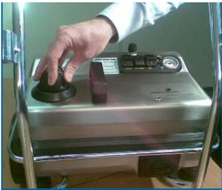
Push down on pressure safety cap then turn the cap anti-clockwise to unscrew.
