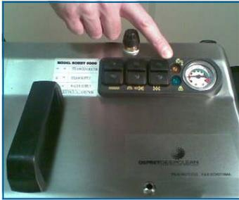
When the low water level light (orange light) lights up: fill up the water tank.
