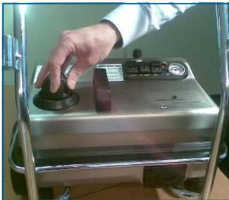
Once the tank is de-pressurised then using **EXTREME CAUTION**: Push down on pressure safety cap then turn the cap
