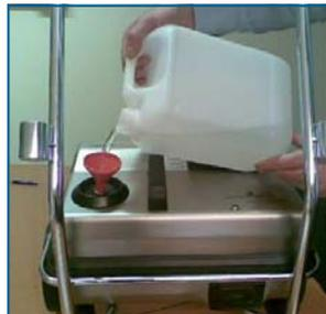
Fill the tank with water using the funnel : **max. 4 ltr.** Preferably hot water. Make sure the tank does not overflow.
