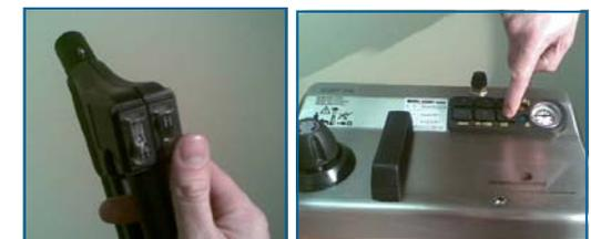
When hot water is required switch on the right switch of the pistol grip and the hot water switch.
