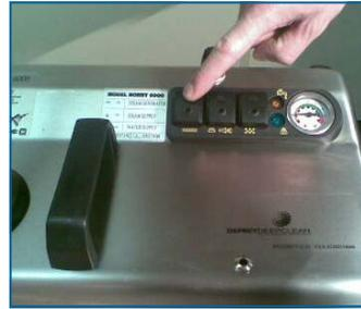
Switch off the machine by using the main switch
