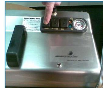
Switch on the main switch. The boiler ready lamp (green lamp) will light up And blink. When the lamp lights up continuously, the machine is ready
