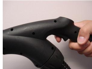
Press the trigger on the pistol grip to release the steam
