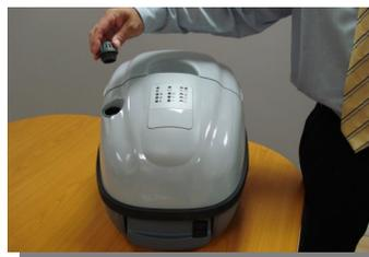
Replace the cap without tightening to much
