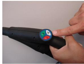
If vacuum is required press the white vacuum switch on the pistol grip. By keeping the switch pressed you move through the three different vacuum levels. When you have reached the vacuum level required, release the white vacuum switch.
