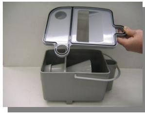
Remove Drum cover sealing element
