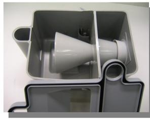
Pour cold tap water into the waste bucket, ensure even level in both compartments
