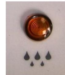
When using detergent and the orange chemical light illuminates; stop operation and refill the chemical tanks
