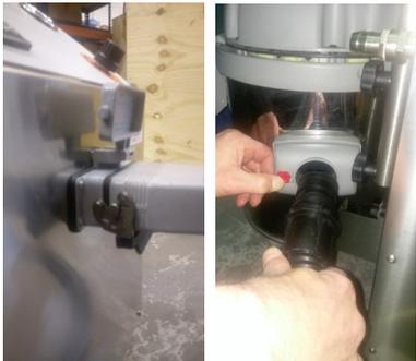
Connect the steam & vacuum hose to the front socket then connect the black vacuum pipe to the vac unit by sliding the red clip to the left. Push the hose into the vac socket and release the red clip to lock in to position
