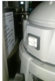
Switch the vacuum unit on using the white switch at the top.
