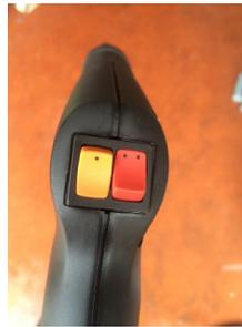
Select the appropriate hose and connect to the front socket. With the steam only hose press the orange button into the ON position. Chemical will be released periodically when the trigger is pressed; releasing the steam
