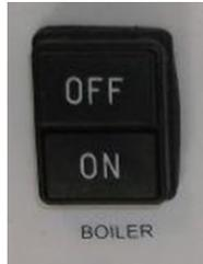
Press the boiler switch button to the ON position and allow the machine to heat up
